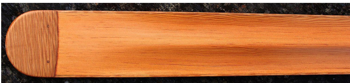
Left hand blade end with scarfed oak tip and edges
