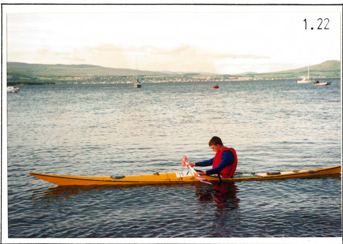
95 LITRES WATER IN COCKPIT (FULL) NEG. No 1.22
