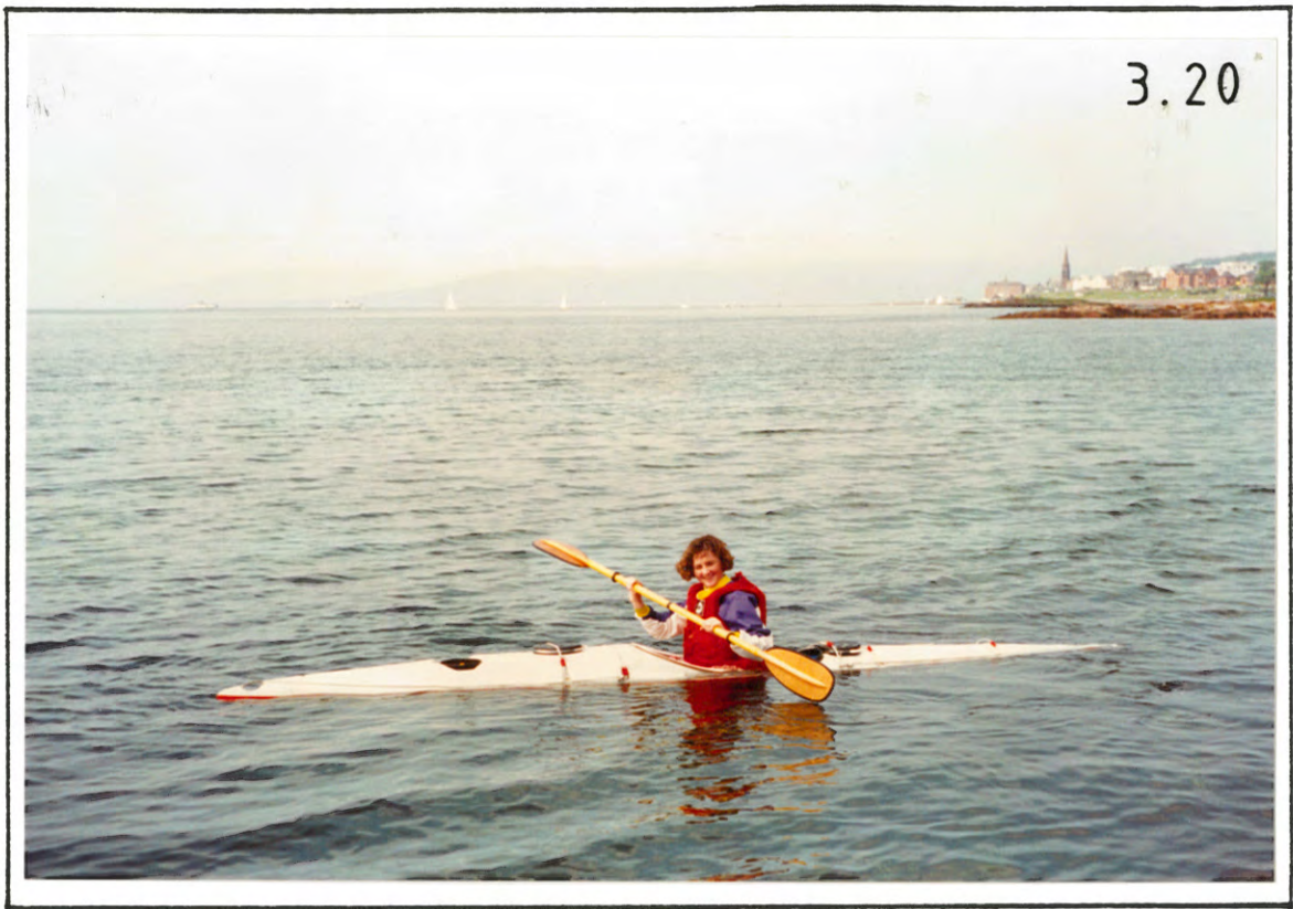
200 LITRES WATER IN HULL, HATCHES OFF, WATER FLOWS IN & OUT AT WILL. NEG. No. 3.20
